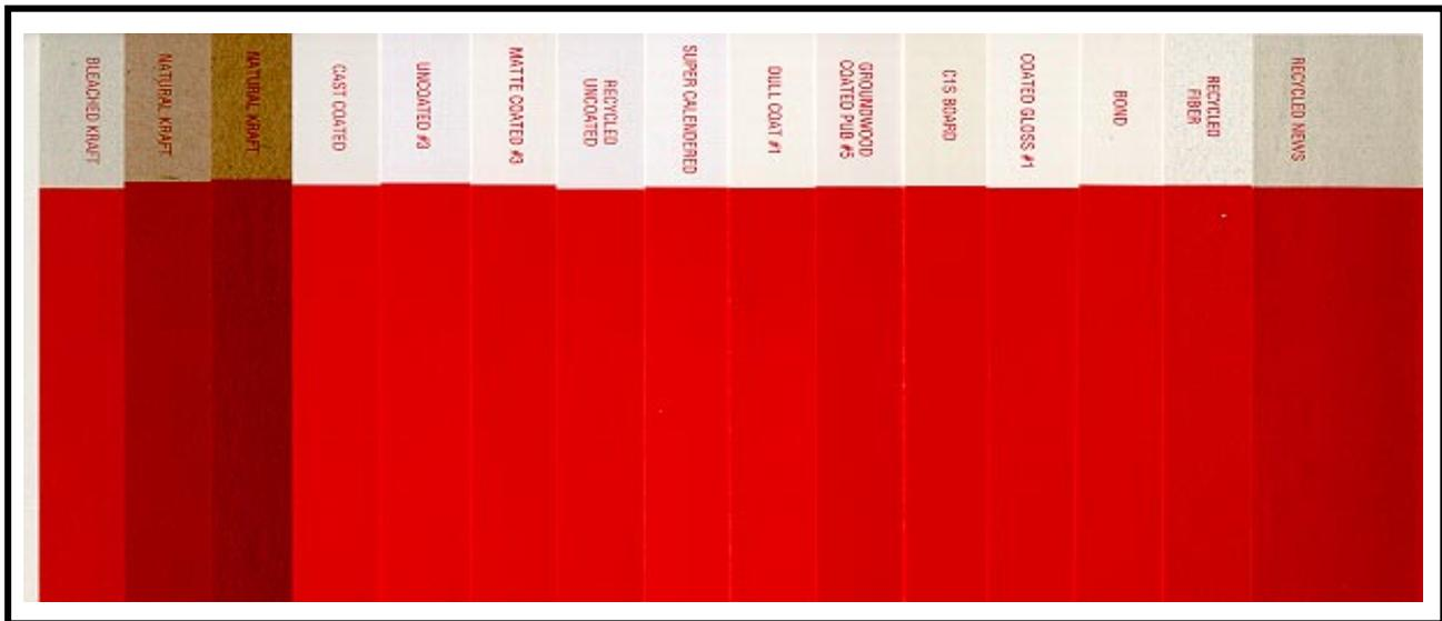
**Whiteness** of a substrate can be defined as the absence of a color or the ability to reflect equal amounts of red, green, and blue light. White sheet is supposed to be a neutral sheet, but in practice most white papers have a slight yellow or blue cast. The substrate should be as neutral as possible in order to avoid printed color distortion.
